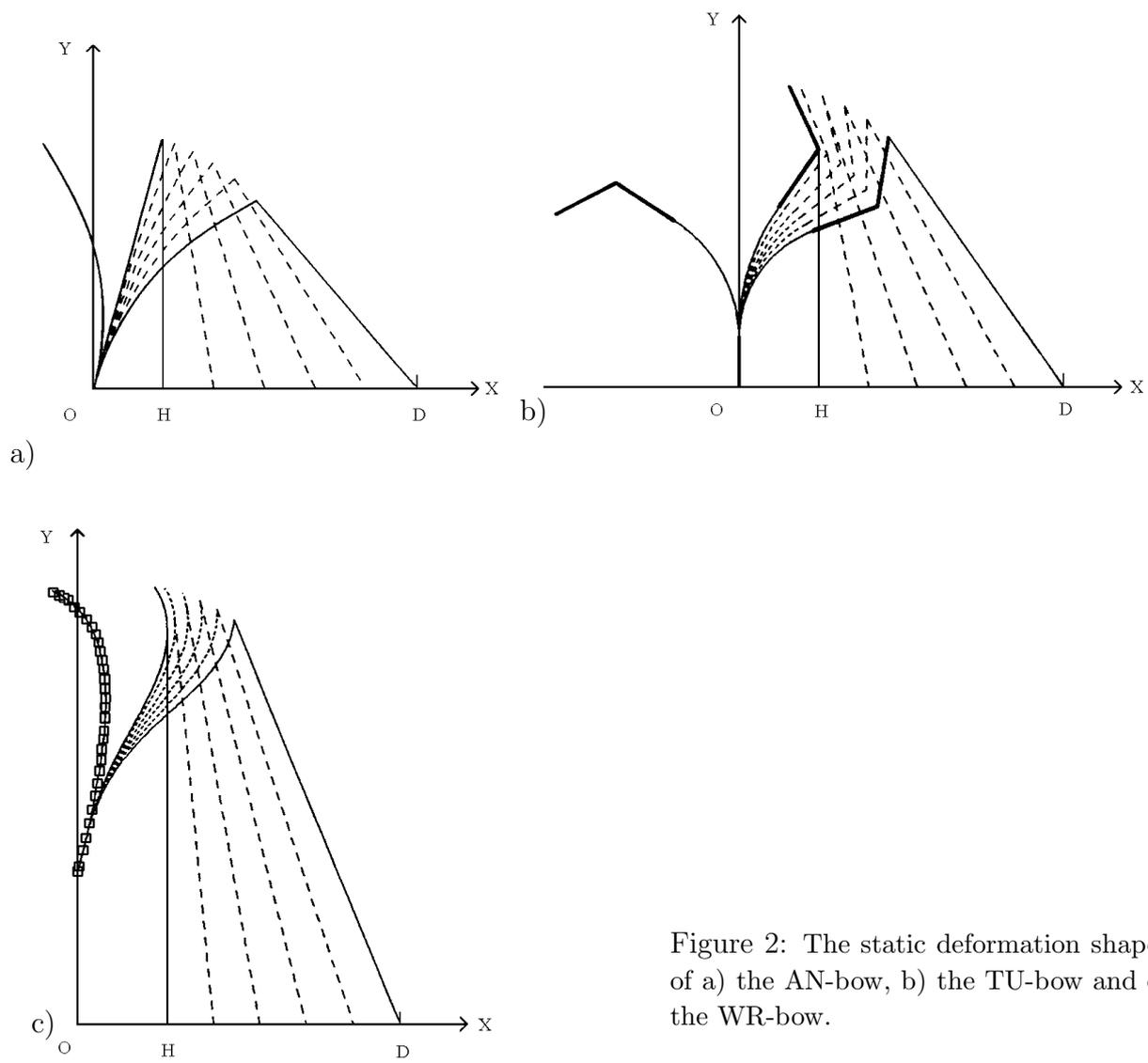
Figure 2: The static deformation shapes of a) the AN-bow, b) the TU-bow and c) the WR-bow.
