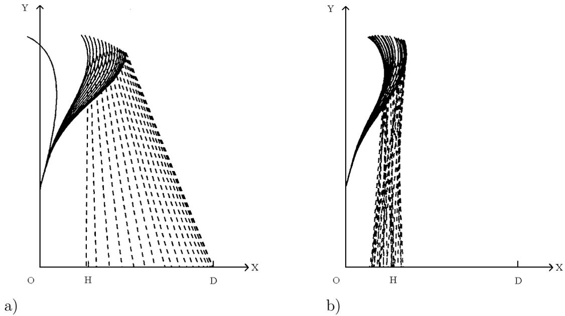
Figure 3: Dynamic deformation shapes of the WR-bow for a)  $0 \leq t \leq t_l$  and b)  $t_l \leq t$ .
