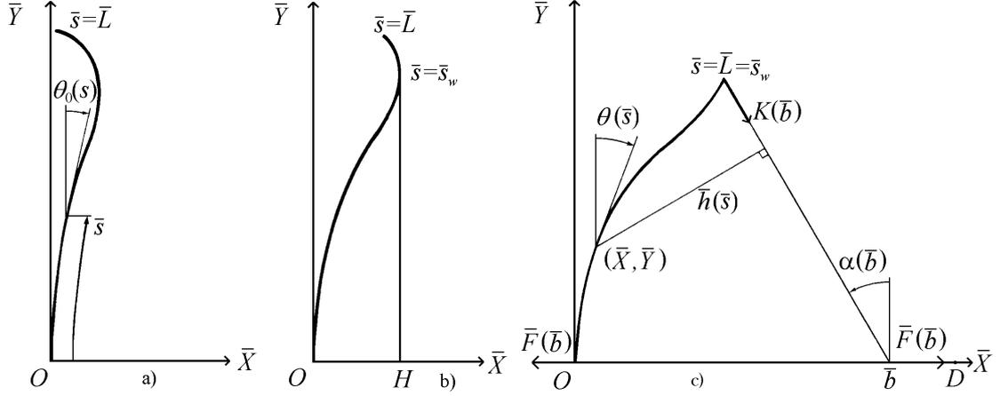
Figure 1: Three situations of the working-recurve bow: (a) unbraced, (b) braced, (c) partly drawn.
