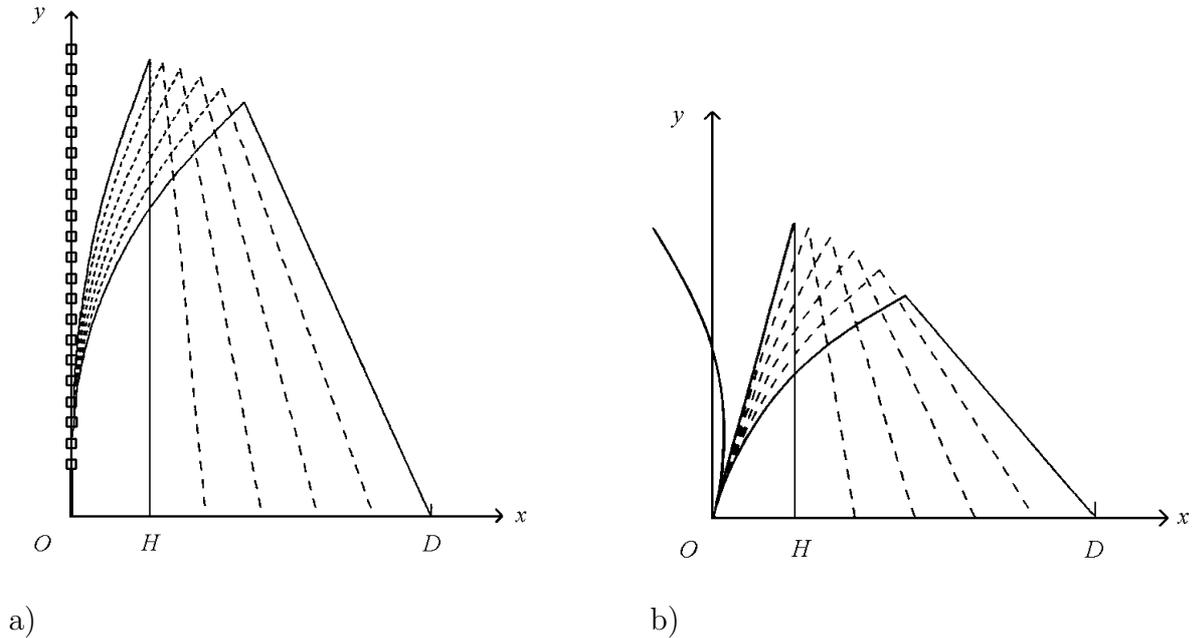
Figure 3: Static deformation shapes (a) of the KL-bow and (b) of the AN-bow.
