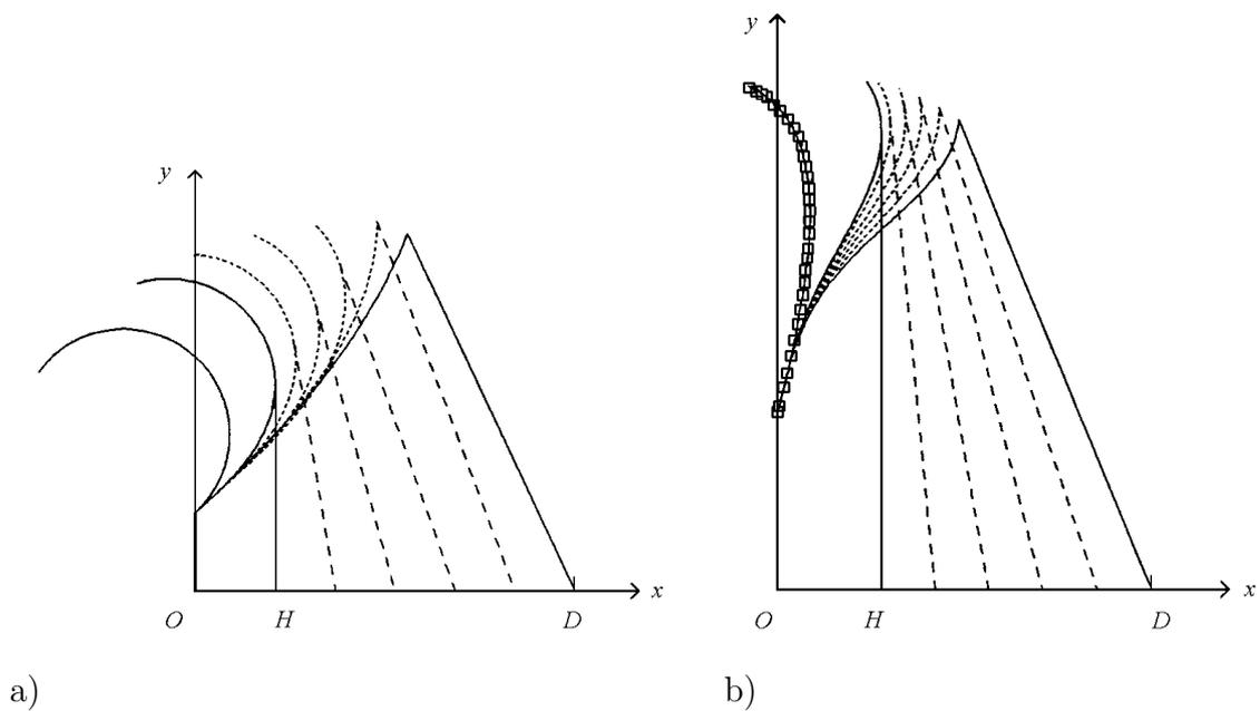
Figure 5: Static deformation shapes (a) of the ER-bow and (b) of the modern working-recurve bow WR-bow.
