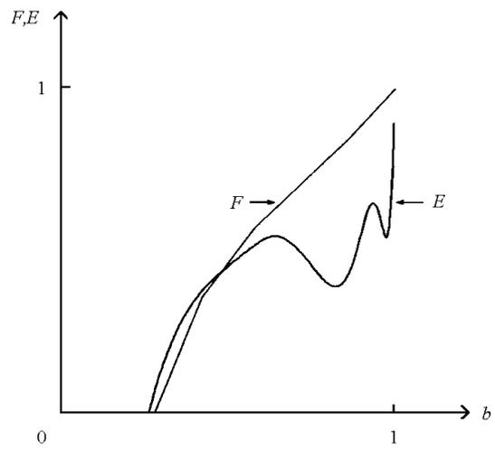
Figure 7: Static Force Draw curve and Dynamic Force Draw curve for the WR-bow.
