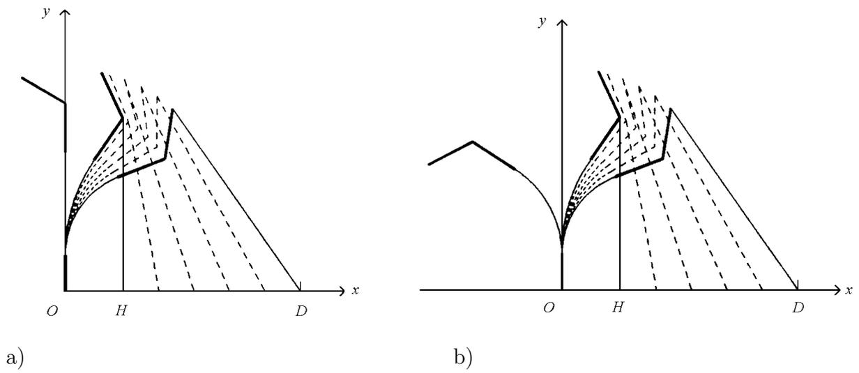
Figure 4: Static deformation shapes (a) of the PE-bow and (b) of the TU-bow.
