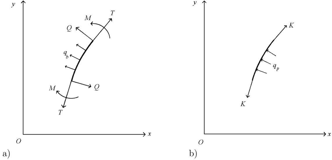
Figure 2: Forces and moments acting upon an element (a) of the limb and (b) of the string.
