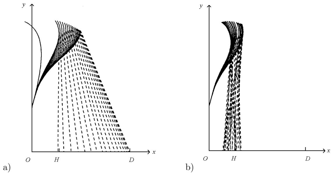
Figure 6: Dynamic deformation shapes of the WR-bow (a) for  $0 \leq t \leq t_l$  and (b) for  $t_l \leq t$ .
