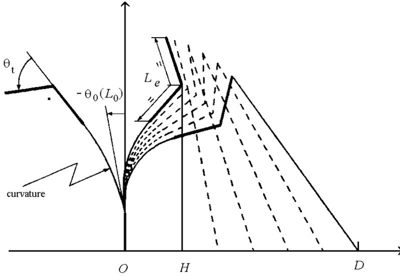
Figure 1: A static-recurve bow in various situations. In this paper I deal with the influence of the parameters,  $\theta_t$ ,  $L$ ,  $L_e/(L - L_0)$  and  $\theta_0(L_0)$  on the performance of the bow.
