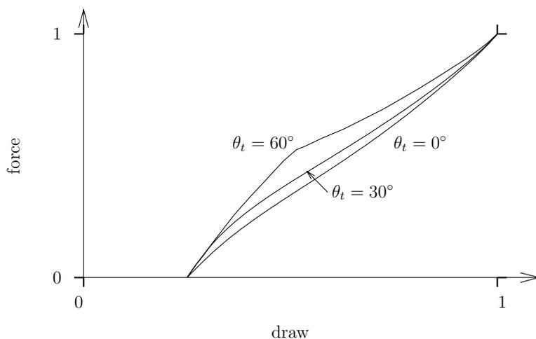
Figure 4: SFD curves for PE-bow with  $\theta_t = 0^\circ$ ,  $\theta_t = 30^\circ$  and  $\theta_t = 60^\circ$  (see also Table 2).
