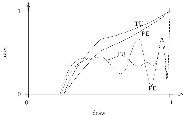
Figure 2: Static (solid line) and dynamic (dashed line) force-draw curves for the static-recurve PE-bow and TU-bow.
