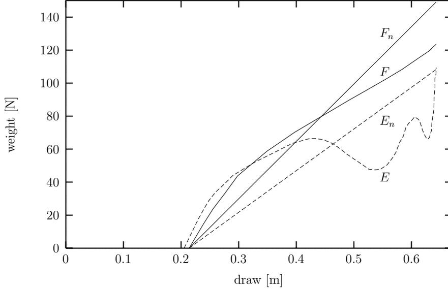
Figure 7: Calculated Static Force Draw curve,  $F$  and Dynamic Force Draw curve,  $E$  for a modern working-recurve bow. The SFD curve  $F_n$  and the DFD curve,  $E_n$  of the associated linear-spring bow used by Pękaliski (1990).
