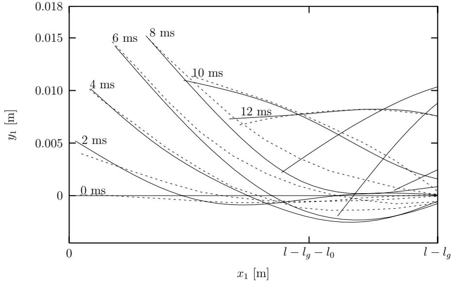
Figure 9: Curves of arrow's deflection on basis of experimental data, dashed line ( --- ) after (Pełkalski, 1990), and on basis of new mathematical model for the arrow, solid line ( — ) every 2 ms after release and for model results until arrow nock passes grip. Acceleration force  $E$  is predicted force shown in Fig. 7.
