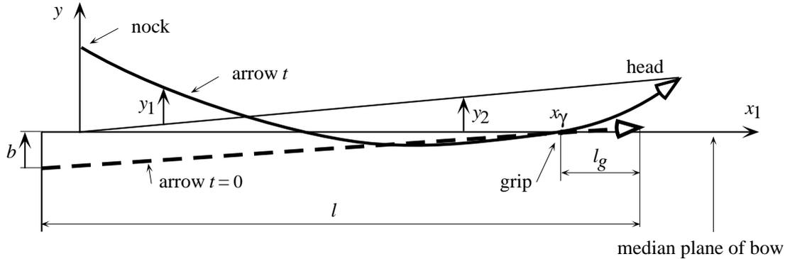
Figure 5: Solid line shows the shape of the arrow, the dashed line is the shape at  $t = 0$ , which is out of the median plane of the bow. The displacement out of the median plane is  $y = y_1 + y_2$ .
