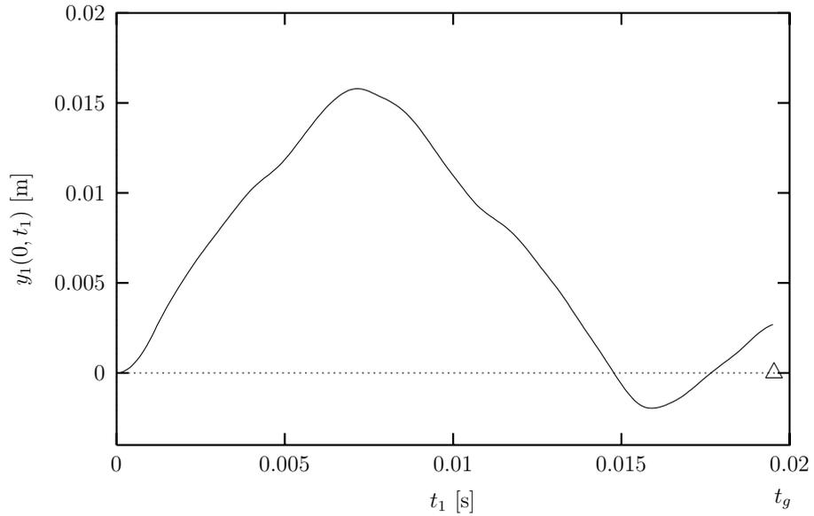
Figure 11: Path of arrow nock for the standard arrow Easton X7 1714 ( $d = 17/64$  inch and  $g = 14/1000$  inch). The acceleration force  $E$  is shown in Fig. 7. At  $t_g$ , indicated by the symbol ‘ $\triangle$ ’ on the  $t_1$ -axis, the arrow nock passes the grip.
