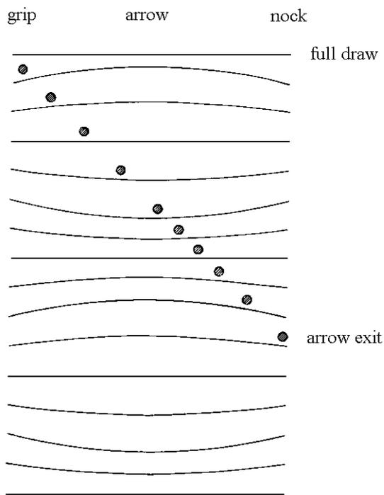
Figure 2: Schematic representation of the phases of the arrow in its passage from the bow, based on evidence from speed-flash photography (after Klopsteg<sup>1</sup>). The shape of the arrow is shown in a coordinate system fixed to the arrow.
