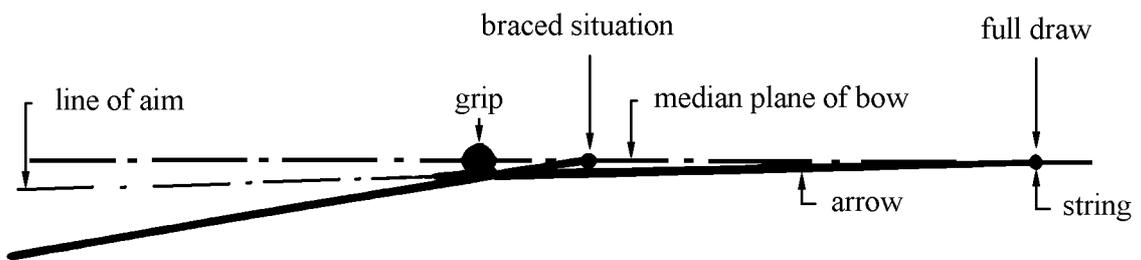
Figure 1: Illustration of the archer's paradox (after Klopsteg<sup>1</sup>). A rigid arrow will change direction as the string gets closer to its equilibrium point in braced position. Therefore it would seem that the arrow should fly far left, since it passes on the left side of the bow.
