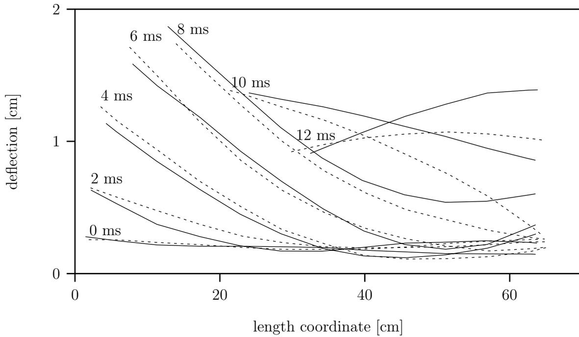
Figure 3: Curves of the measured arrow deflections ( - - - ) and the arrow deflections predicted by Pękal'ski's mathematical model ( — ) every 2 milliseconds (ms) after release (after Pękal'ski<sup>17</sup>). The shape of the arrow is shown in a coordinate system fixed to the bow; the arrow in the fully draw position is the line at 0 ms and the place of the grip of the bow is close to the bottom right corner.
